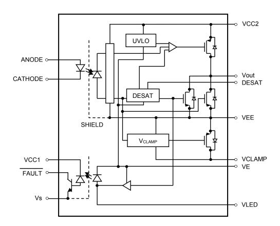
Note: A  $1-\mu F$  bypass capacitor must be connected between pins 9 and 13, pins 13 and 16.
