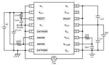
$\mathsf{CML}\ (\mathsf{CMH})$  is the maximum rate of rise (fall) of the common mode voltage that can be sustained with the output voltage in the LOW (HIGH) state.
