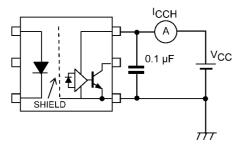
Fig. 13.1.3 I<sub>CCH</sub> Test Circuit
