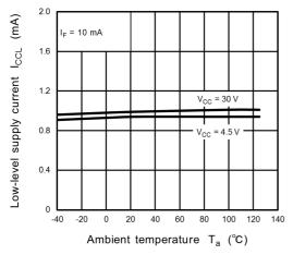
Fig. 13.2.5 I<sub>CCL</sub> - T<sub>a</sub>
