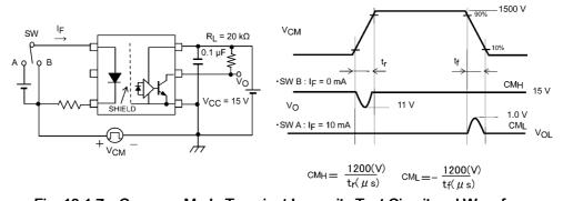
Fig. 13.1.7 Common-Mode Transient Immunity Test Circuit and Waveform
