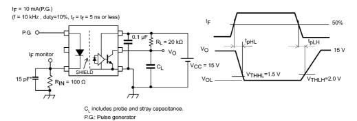
Fig. 13.1.6 Switching Time Test Circuit and Waveform
