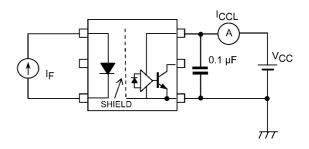
Fig. 13.1.4 I<sub>CCL</sub> Test Circuit
