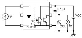
Fig. 13.1.2 V<sub>OL</sub> Test Circuit
