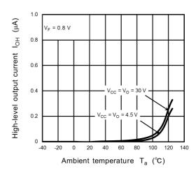
Fig. 13.2.4 I<sub>OH</sub> - T<sub>a</sub>
