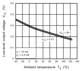
Fig. 13.2.8 V<sub>OL</sub> - T<sub>a</sub>
