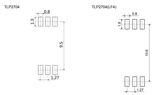
Fig. 15.1 Lead Forming Option (standard)
