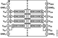
Figure 2. ADuM1401 Functional Block Diagram
