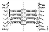
Figure 3. ADuM1402 Functional Block Diagram
