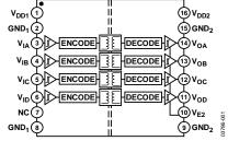
Figure 1. ADuM1400 Functional Block Diagram
