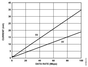
Figure 14. Typical ADuM1401  $V_{\rm DD2}$  Supply Current vs. Data Rate for 5 V and 3 V Operation
