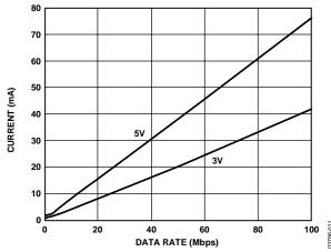
Figure 11. Typical ADuM1400 V<sub>DD1</sub> Supply Current vs. Data Rate for 5 V and 3 V Operation
