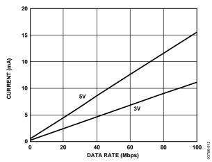
Figure 12. Typical ADuM1400  $V_{\rm DD2}$  Supply Current vs. Data Rate for 5 V and 3 V Operation
