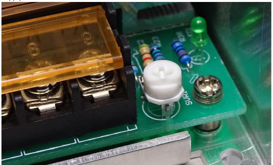
7 RD60xx assembly: If you have CR1220 battery, please install the battery with the positive side facing up, if you have WiFi module, please install it like what shows in the picture. Install RD60xx to the front side in the correct way, otherwise it cannot be installed properly, we make flame tight to prevent the RD60xx from shaking, if the case is slightly deformed, you can gently bend the case to make it straight.
