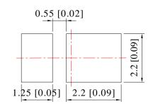
Unit: mm Tolerance: ±0.10mm
