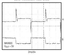
A: OUTPUT VOLTAGE (100mV/div) B: I<sub>OUT</sub> = 500mA (HIGH), I<sub>OUT</sub> = 5mA (LOW)
