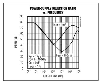
Figure 7. Power-Supply Rejection Ratio vs. Ripple Frequency
