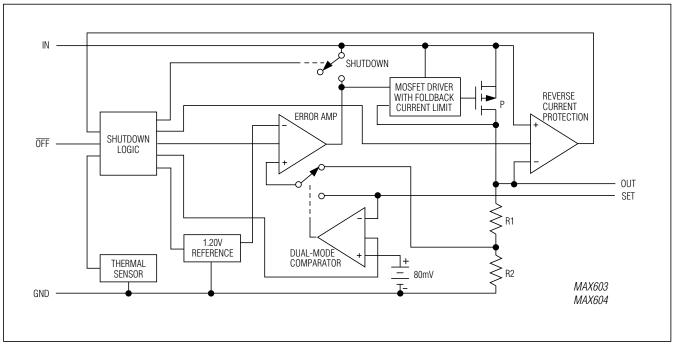
Figure 2. Functional Diagram
