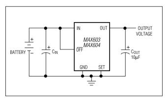
Figure 6. 3.3V or 5V Linear-Regulator Application
