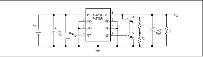
Figure 1. Test Circuit
