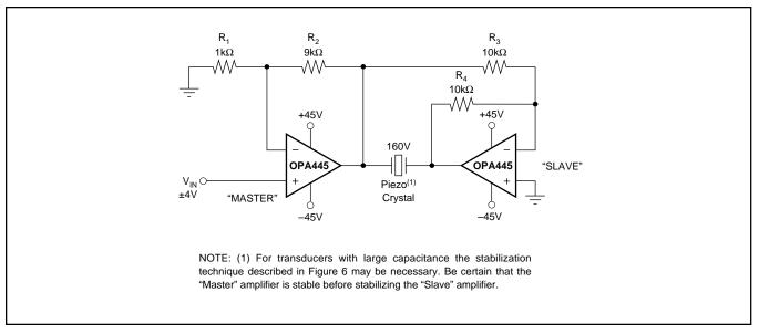
FIGURE 11. Bridge Circuit Doubles Voltage for Piezo Crystals.
