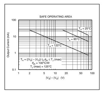
FIGURE 3. 8-Pin DIP Safe Operating Area.
