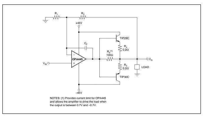
FIGURE 8. External Output Transistors Boost Output Current up to 1 Amp.
