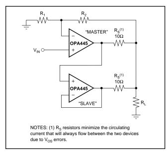
FIGURE 7. Parallel Amplifiers Increase Output Current Capability.
