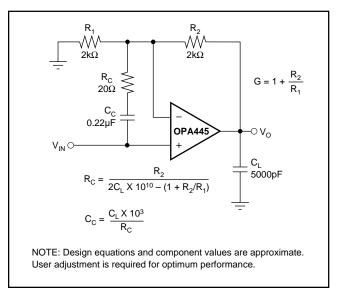
FIGURE 6. Driving Large Capacitive Loads.
