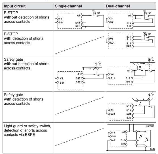
The E-STOP pushbutton and safety gate switch symbolise a trigger element with N/C / N/C combination.
