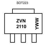
ZVN2110 = Product Type Marking Code YWW = Date Code Marking Y or  $\overline{Y}$  = Last Digit of Year (ex: 5= 2015) WW or  $\overline{W}W$  = Week Code (01~53)
