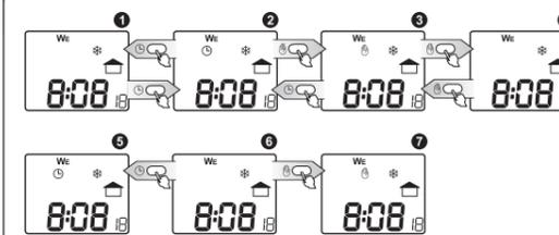
The manual op mode change (the bell manual switching ON / OFF) – if the main window is open and the automatic mode is set 1 pressing the key ⌚ will cause entering the manual mode 2; successive key ⌚ pressing will cause changeover between 3 & 4 the manual mode and the OFF mode..
