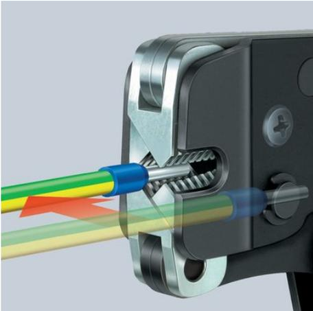
97 53 08: lateral loading of wire ferrules up to 2.5 mm<sup>2</sup> parallelly from the side e.g. in confined areas
