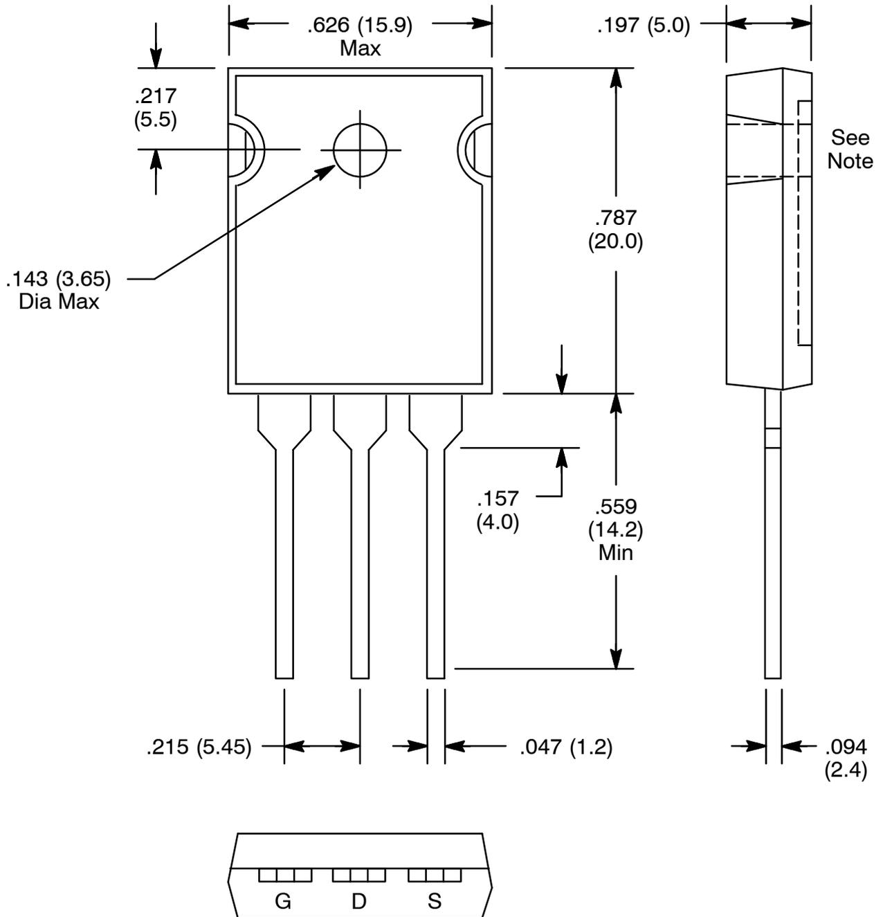
**Note:** Drain connected to metal part of mounting surface.
