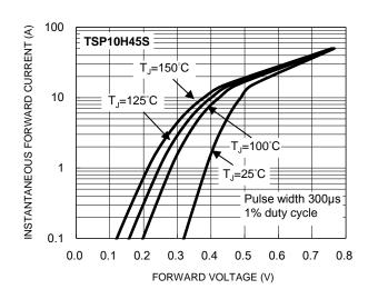
Fig.6 Typical Forward Characteristics
