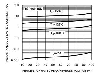
Fig.5 Typical Reverse Characteristics
