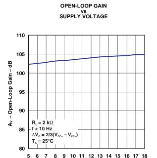
V<sub>cc+</sub>/-V<sub>cc-</sub> - Supply Voltage - V
