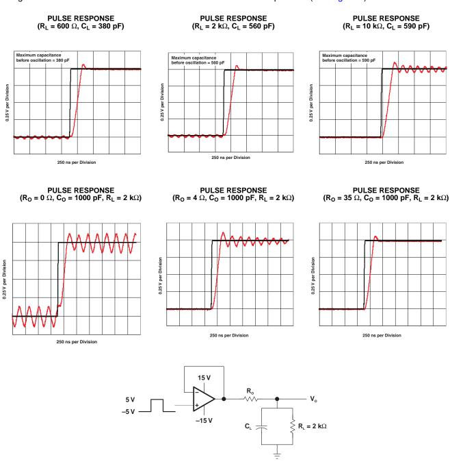
Figure 2. Output Characteristics
