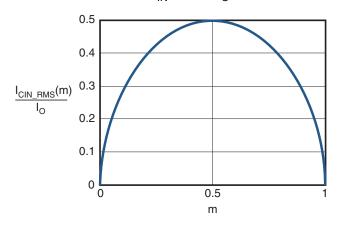
Figure 2. I<sub>CIN</sub> vs. Voltage Conversion Ratio
