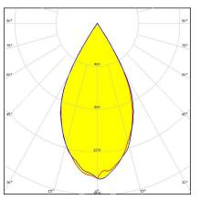
Dimensions: 182.0 mm x 40.0 mm Height: 20.20 mm ~50° beam. 4X1 variant.
