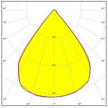
Dimensions: 182.0 mm x 40.0 mm Height: 20.20 mm ~80° wide beam. 4X1 variant in white.
