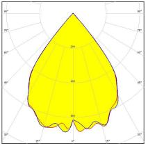
Dimensions: 182.0 mm x 40.0 mm Height: 20.20 mm ~80° wide beam. 4X1 variant.
