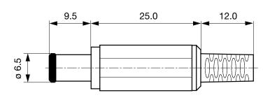
Cable diameter max. 4.0 mm
