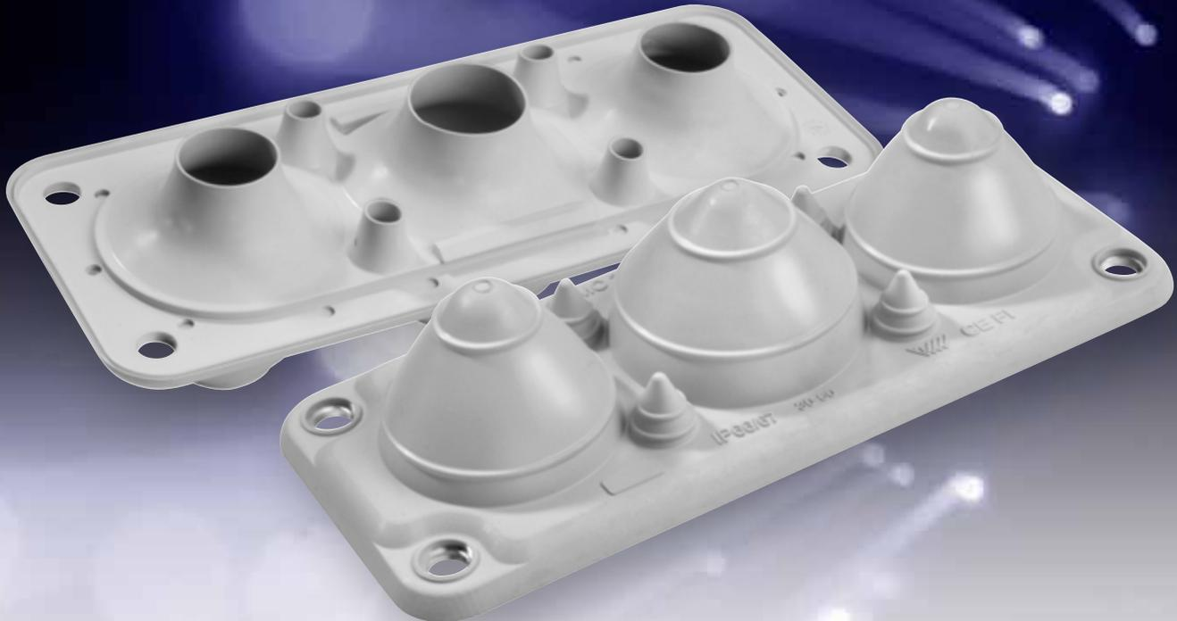
MC 3/7 Multigate is suitable for leading through both low and medium power current cables as well as various types of tubing. It fits directly to a C-standard cut-out (or FL 21).
