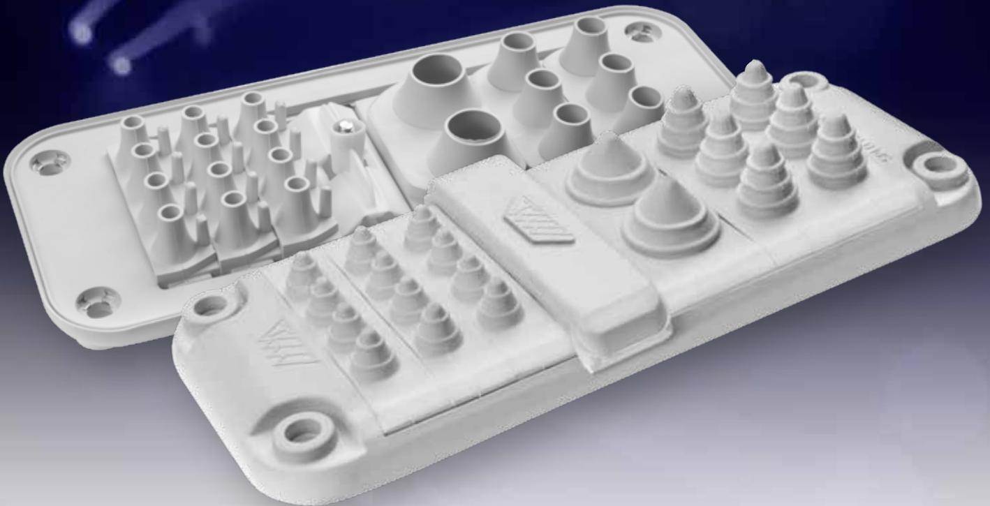
Splitting Multigate is based of totally new philosophy and is provided for cables with connectors or/and without. Splitting Multigate is metal and plastic reinforced cable gland plate combination for leading through both low and medium power current cables as well various types of tubing and it wires. The product fits directly to c-standard cut-out ( FL 21 ).
