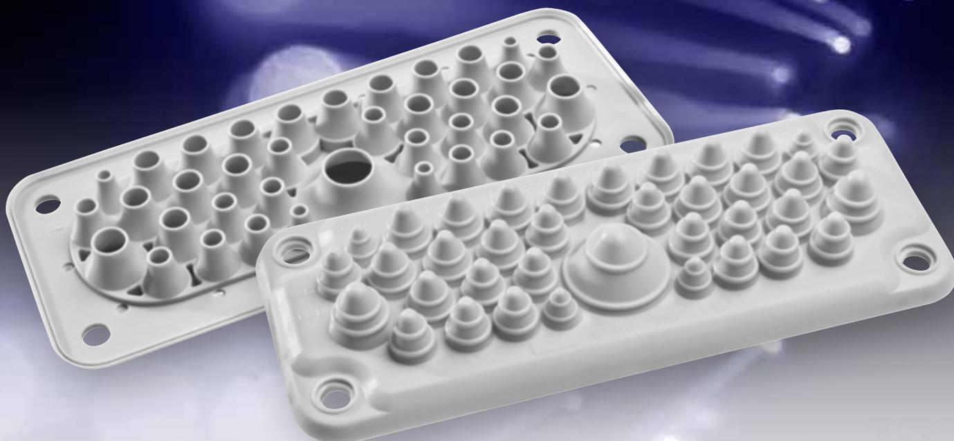
MC 35/37 Multigate is suitable for leading through both low and medium power current cables as well as various types of tubing. It fits directly to a C-standard cut-out (or FL 21).
