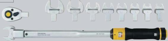
The open-end spanners enable lateral access for tightening screws and sleeves on pipe connections, hydraulic systems and threaded rods. Automatic quick release: Clearly audible and palpable click signal when selected torque is reached. Piece by piece calibration and inspection for high accuracy according to ISO 6789 (+/- 3 %). Plugon tools with square joint (14 x 18mm) to safely lock into position
